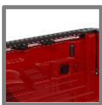
Trail Rail: a system of sturdy hooks on guides for better control of cargo
